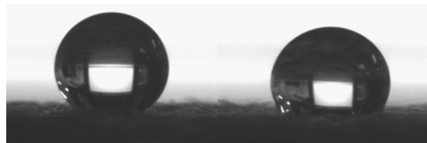
Fig. 5 10 \mu L water (left) and hexadecane (right) droplets sitting on top of NyCo treated with FS via microwave synthesis
